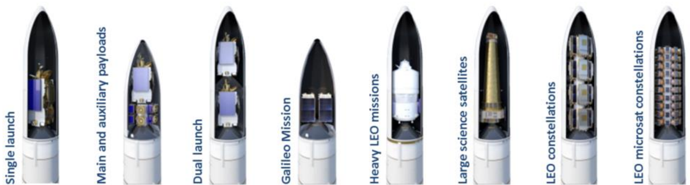
Ariane 6 possible missions and configurations | Photo: ESA
